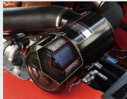
Optimized air intake and exhaust system of full vehicle, high-capacity exhaust silencer and high-effect intake silencer will reduce the noise of full vehicle and reduce the vibration.
